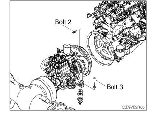
③ Using a moving truck slowly pull out transmission assembly to the front.
